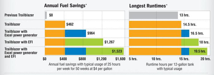
\*Based on typical usage — 150 amps welding 40% of the time; 20 amps generator power 30% of the time; and idling without load 30% of the time.
